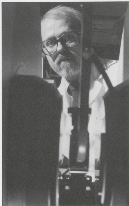
Allan Butterfield, director of the Center of Membrane Sciences, examines the sample cavity between the two poles of the large electromagnet used in conjunction with an electron spin resonance spectrometer. This equipment is used to investigate membrane structure and function.
