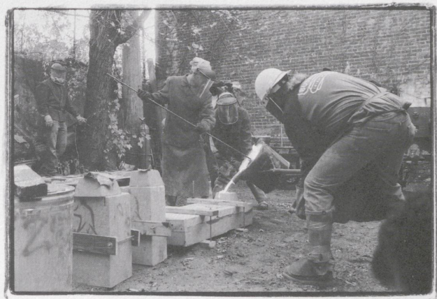
POURING MOLTEN IRON IN RESIN SAND MOLDS
