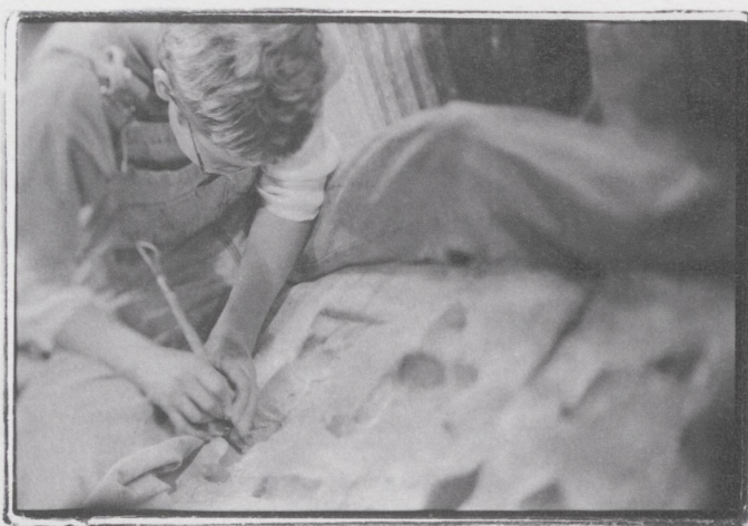
TERESA KOESTER, A GRADUATE ASSISTANT IN ART, PREPARES A RESIN SAND MOLD.
