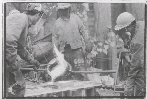
JERRY MASSE (LEFT) SKIMS SLAG FROM THE TOP OF THE MOLTEN IRON TO KEEP IMPURITIES OUT OF THE MOLD.
