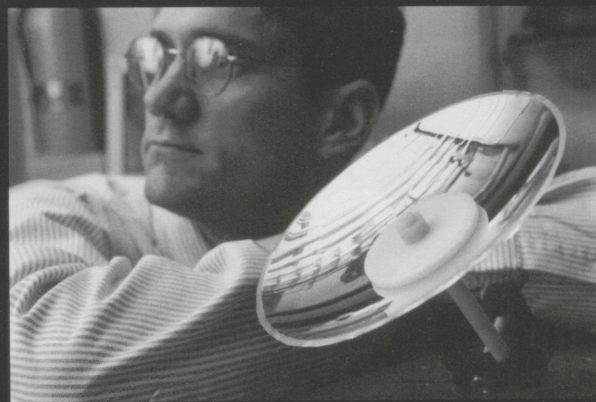
A MYLAR MOCKUP OF THE MIRROR JOHN MAIN IS BUILDING RESEMBLES A MINIATURE SATELLITE DISH MADE OUT OF SHINY METALLIC FILM.
