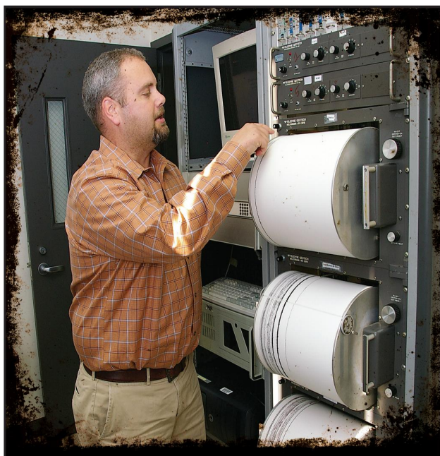
Jonathan McIntyre shows the traditional helicorders recording seismic activity. Today data is sent from the field to UK computers.
