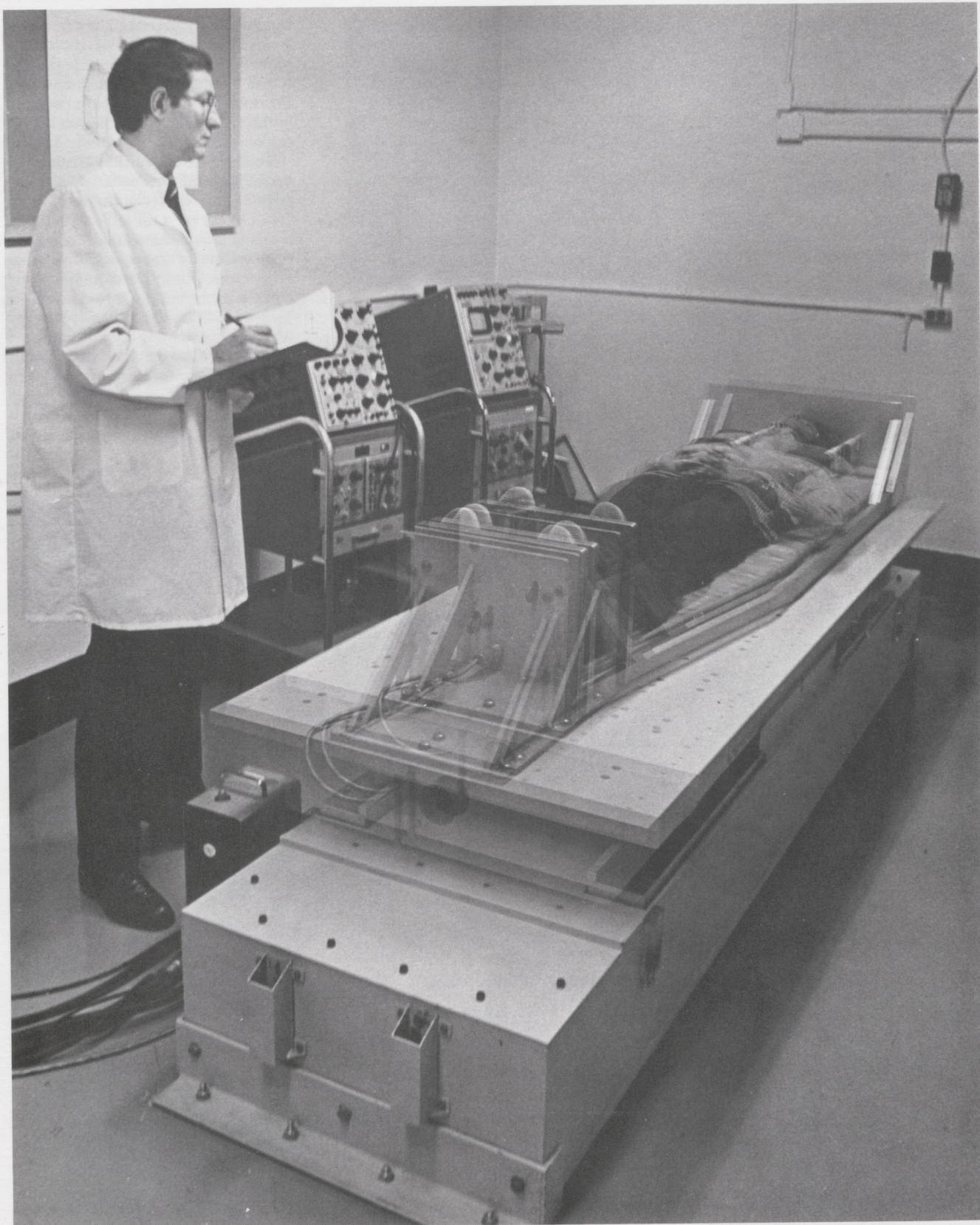
This oscillating platform (also known as "the shake table") is used in research by Dr. Knapp for applications in the deconditioning of space travellers.
