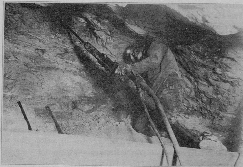
FIGURE 26.— DRILLING IN CRAMPED QUARTERS WITH A WET STOPER The hazards of rock drilling are increased when work is done in restricted space and under difficult conditions.
