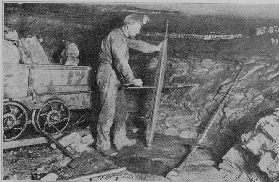
FIGURE 1.— DRILLING WITH A HAND AUGER
